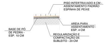
**DETALHE DE PISO INTERTRAVADO S/ ESCALA**
