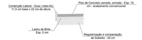
**DETALHE DE PISO DE CONCRETO S/ ESCALA**
