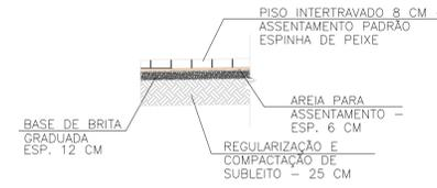
DETALHE DE PISO INTERTRAVADO S/ ESCALA
