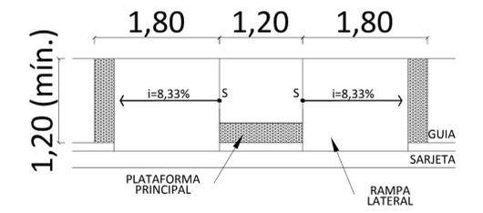
**DETALHE DE RAMPA DE ACESSIBILIDADE SEM ESCALA**
