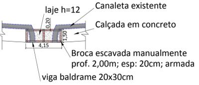
DETALHE DO MURO DE ARRIMO
